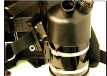
*Those divers that are using a different wing/harness or BCD system, should pay attention to where they place the mounting bracket. On the system that we sell, the mount is located on the lower band. With this system, the mount is in the best position if the top band is placed as close to the top curve as possible. (where the writing is usually stamped) The bands on other systems may not be spaced the same. Our system has approximately 6.5 inches in between the bands.*
