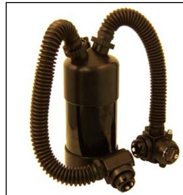
Now the remaining two loop hoses can be attached. These are the hoses with the stainless steel ballast rings. They will have the quick disconnect hose stubs on one end and the mouthpiece hose attachments on the other. These two hoses are identical. Attach the quick disconnect hose stubs to the end of each T-Piece. Ensure that the O-rings on the hose stubs have been lubricated. As per the warning above, ensure that the O-rings have not been pinched. See photos below.
