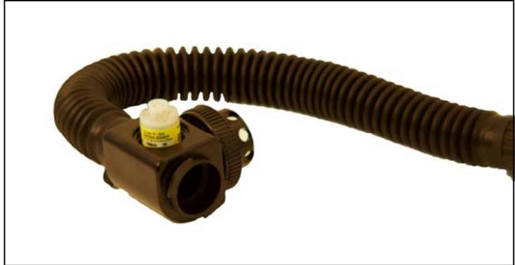
After you have taken the sensor from its bag, and it has had sufficient time to “wake-up”, it can be installed into the GEM diving system. First remove the O-ring on the sensor. It is not required and will also prevent the sensor from being inserted all the way into the T-piece. Once the O-ring on the sensor has been removed, screw the sensor into position . See photo right.
