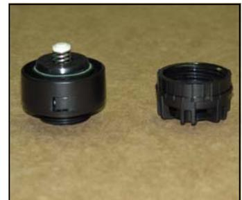
Once the valve is open, you will see a small white button sitting on top of the spring. Carefully remove the button and set it aside (remember which way it came out). Remove the spring and stretch it out a slight amount and then replace it. Re-insert the button, replace the top of the valve and tighten.
