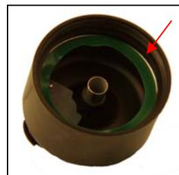
Your scrubber head is now prepared. Prior to diving, divers should ensure that the O-ring is clean and lubricated; that the gasket is in good condition; the OPV is tightened all the way down; the towers are not damaged.
